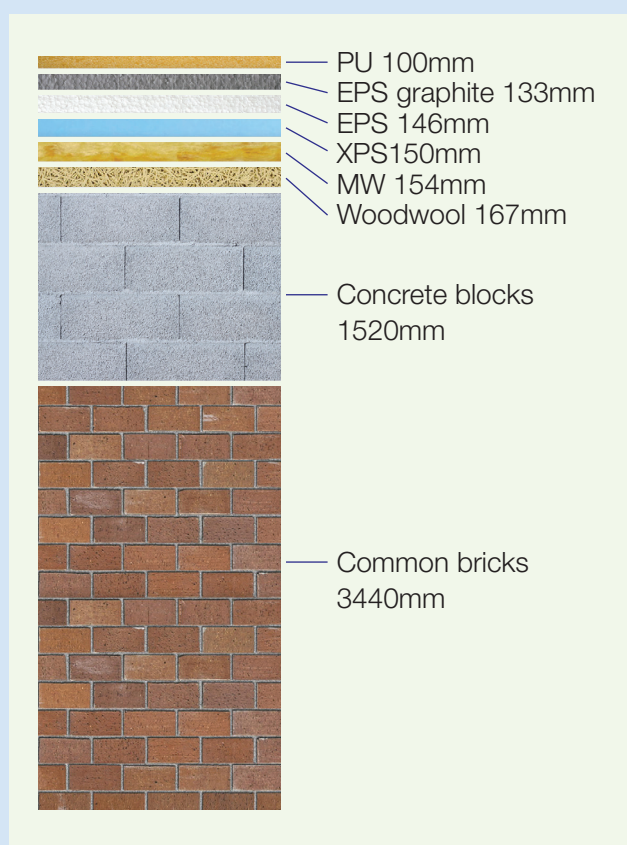
Figure 2: Insulation thickness at equivalent R-value.
